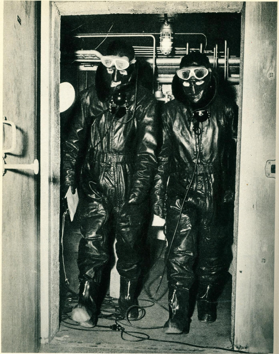
The Cold Room, sometimes referred to as the Boeing LABRRRRatory, where temperatures as low as -80 F. can easily be reached and held indefinitely.
